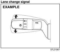
Move the lever part-way in the direction to turn and hold it there.
